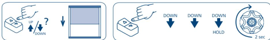
Using the button to be linked to ascent bring the awning up to the desired position (for cassette-awnings, hold the button pressed until the motor stops automatically on the closing position).
