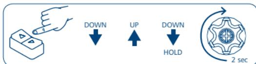
Press the buttons as indicated in rapid sequence and hold the button
